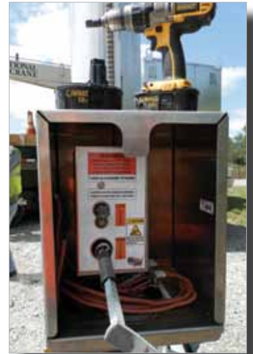
Can be raised and lowered manually (hand-crank) or via a power drill
