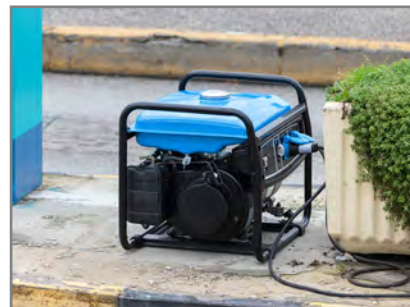
Typical gas/diesel generators require refueling intervals of every 8-10 hours to remain operational during times of crisis.
